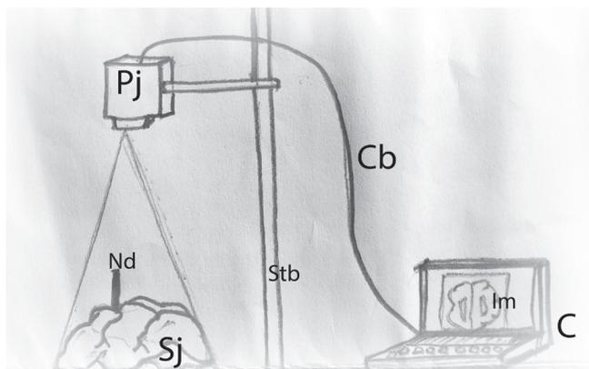
**Figure 1.** In this figure, the experimental procedure was schematized. The virtual image was projected over the specimen to localize the frontal horn of the lateral ventricle before inserting a needle. (Pj: projector, Nd: needle, Sj: subject, Stb: stabilizer, Cb: cable, Im: image, C: computer).
